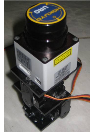
Fig. 2. LASER Range finder is mounted on a stabilizing mechanism. This mechanism keeps the LASER range finder horizontal on roll-pitch ramps. A 3DOF gyro is used to sense roll and pitch values.
