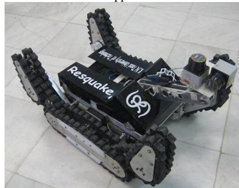
Fig. 1. Silver, the experimental platform of this research, with two LASER range finders installed on its passive robotic arm
