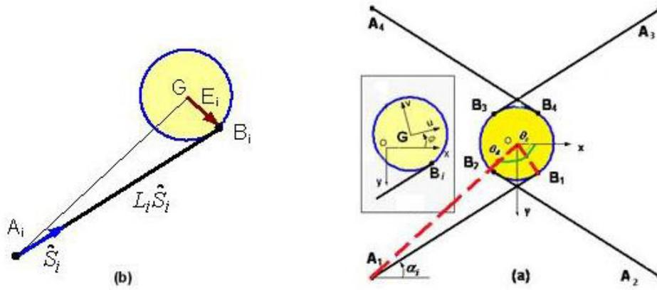
Figure 1: (a): The schematics of planar cable mechanism (b): Vector definitions for jacobian derivation
