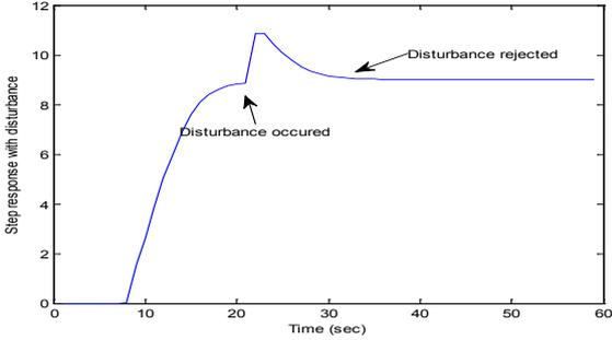
Figure 2. Set point and disturbance response
