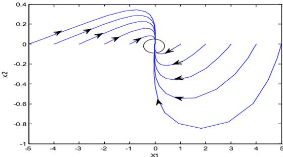
Figure 4. phase portrait of closed loop near the origin
