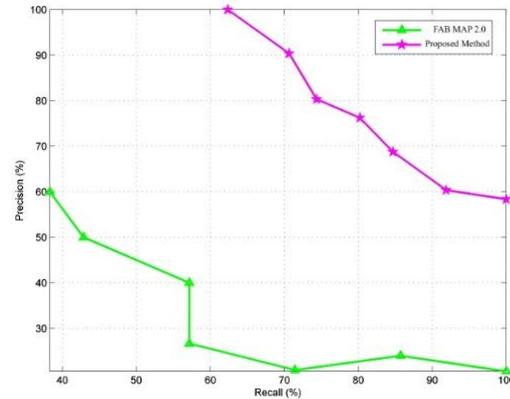
Figure 6: The precision-recall curve of KITTI Sequence (00).
