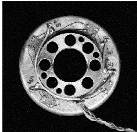
FIGURE 5. Harmonic drive built-in torque sensor
