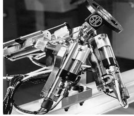
Figure 2. The hydraulic shoulder in movement
