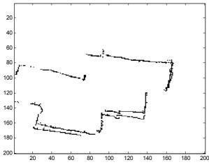
Figure 5 – Global map when the robot move around the room
