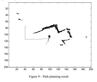
In Figure 9 the initial robot direction is shown by an arrow to determine the robot orientation. Unexpanded walls are shown in as a black areas and obtained path is shown in gray line.
