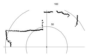
Figure 4 - Pre-filtered data of the LRF, noise has been omitted
