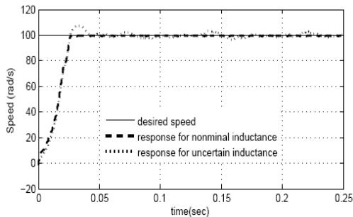
Figure 6. Estimated speed for 70% uncertainty in stator inductance
