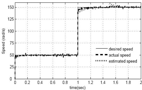
Figure 1. Speed reference, estimated and actual speed responses
