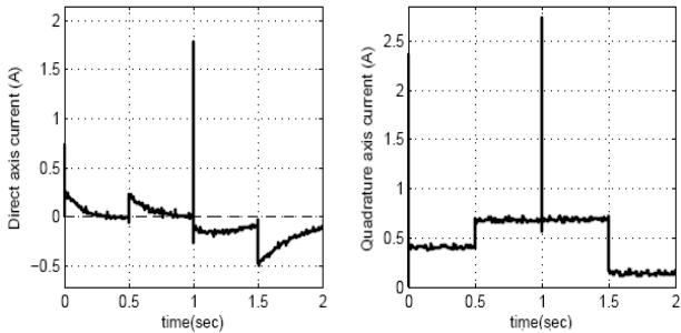
Figure 2. Actual direct and quadrature axis currents
