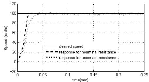
Figure 5. Estimated speed for 50% uncertainty in stator resistance
