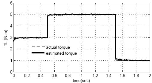
Figure 4. Actual and estimated load torque
