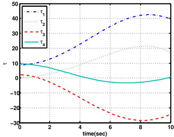
Fig. 5. The projection of the moving platform forces on actuators.
