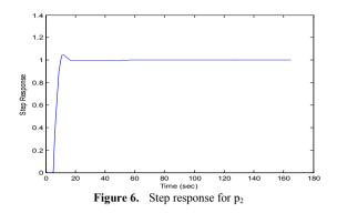
This example shows that the closed loop system is strictly proper regardless of any bounded model uncertainties. Moreover, it provides an example of robust stability and zero frequency performance design.
