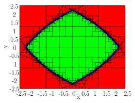
Fig. 8 Point-displacement FKS, the inside(green) region, of a 4-RPR with  $c=\infty$  and f=2 and  $\sigma_d=0.3$  with  $\phi=\frac{\pi}{6}$ . The dashed lines represent the boundary of the workspace.
