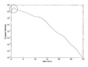
**Fig. 4.** The values of the Lyapunov function (33) of the proposed robust SDRE filter for large initial error.
