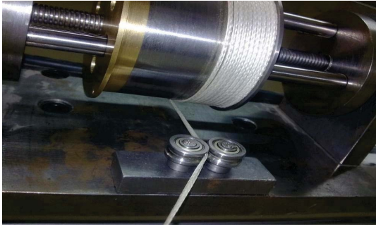
Fig. 5. The system of cable winch
