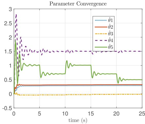
Fig. 6: Parameter estimation of master #1 Manipulator
