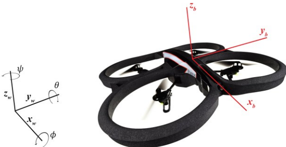
Fig. 1. AR. Drone (body) coordinate system and world coordinate system.
